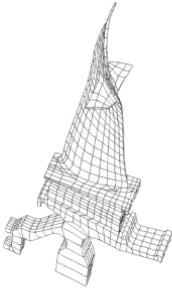
Figure 6: 1T Modeshape (1 T) of the first rotor blade of a multi-stage high pressure axial compressor
