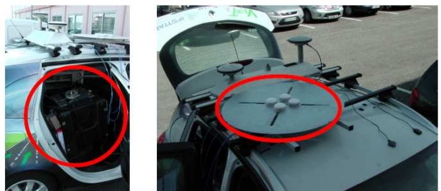
Fig. 3: Bit Grabber (left) and antenna array (right) mounted on a car.
