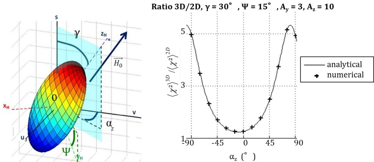
Figure 1. Left: high latitude configuration of anisotropy ( $\vec{H}_0$  representing earth magnetic field), in blue the 2D cut plane of 3D to 2D reduction. Right: 3D to 2D log-amplitude variances ratio versus  $\alpha_z$  angle.
