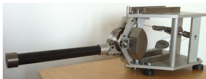
Figure 9. 1-DOF prototype robot integrating a differential cable drive actuator.
