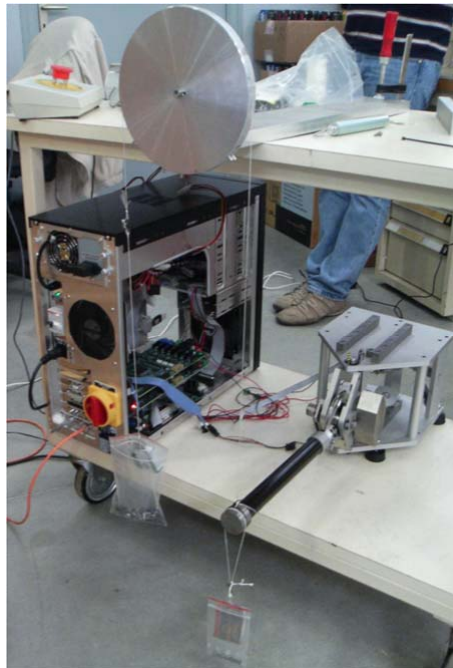
Figure 10. Configuration used to measure the differential cable drive actuator's friction.
