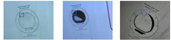
Figure 9: Air inlet vent - sliding window inspection.
