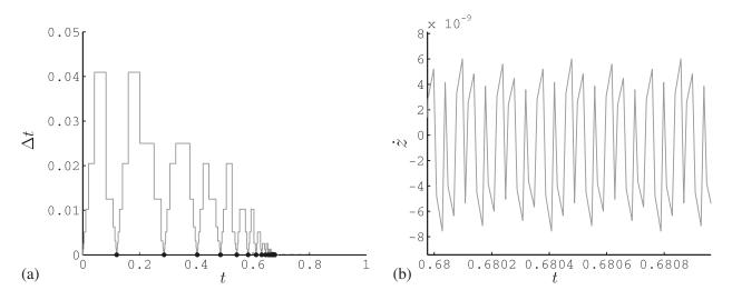
Figure 9. Simulation results of a point mass falling on a table. Computations have been done *without* the restriction of using only an uneven number of extrapolation substeps: (a) the time evolution of the step size  $\Delta t$  and (b) high-velocity oscillations that prevent the step size from being increased.
