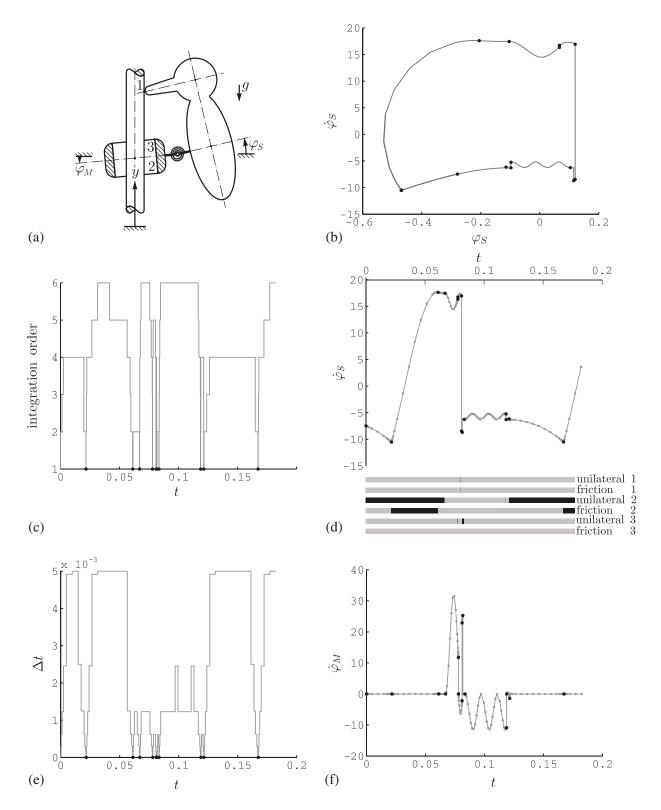
Figure 13. Woodpecker toy together with the results of the simulation. The time evolutions of  $\dot{\phi}_M$  and  $\dot{\phi}_S$  are complemented by a diagram, which shows the discrete state  $\hat{\sigma}$  of the six different set-valued laws. Black parts correspond to the 'constraint' mode; grey parts correspond to the 'impressed' mode.
