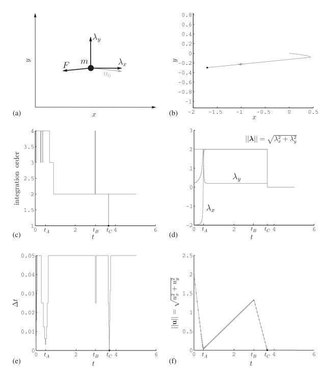
Figure 11. Point mass sliding on a table. (b) The path in the *xy*-plane. (c)–(f) The time evolutions of the integration order, the step size  $\Delta t$ , the friction force  $\lambda$  and the absolute velocity of the point mass. At time instants  $t_A$ ,  $t_B$  and  $t_C$  the point mass turns around, the force is switched off and a slip-stick transition occurs, respectively.
