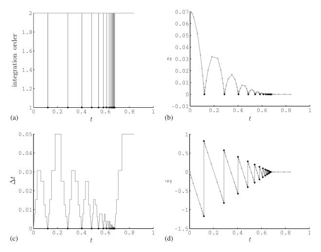
Figure 10. Simulation results of a point mass falling on a table. (a)–(d) The time evolution of the step size  $\Delta t$ , the integration order, the height z and its derivative  $\dot{z}$ .
