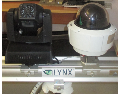
Figure 1: Acquisition system : PTZ camera and the directional light device
