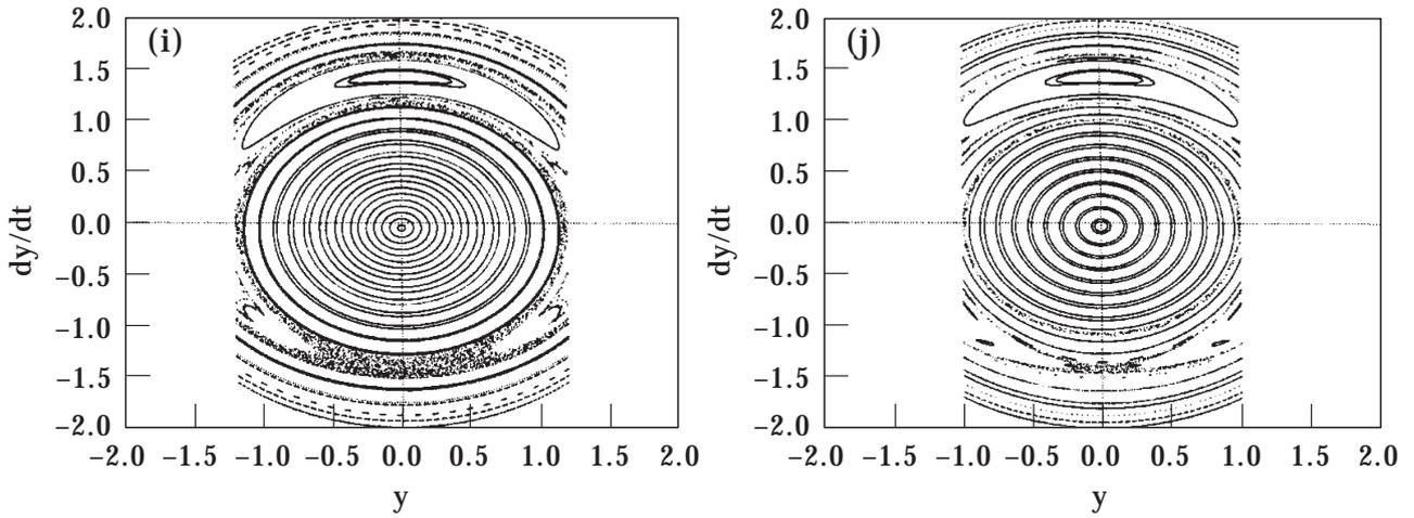
Figure 8. Global Poincaré map of the system with  $\alpha = 1$ ,  $\beta = \delta = 0$ ,  $\gamma = 0.1$  and energy  $h = 2$ , for clearances: (a)  $e = 2.0$  (no impacts), (b)  $e = 1.9$ , (c)  $e = 1.88$ , (d)  $e = 1.85$ , (e)  $e = 1.8$ , (f)  $e = 1.78$ , (g)  $e = 1.5$ , (h)  $e = 1.4$ , (i)  $e = 1.2$ , (j)  $e = 1.0$ .
