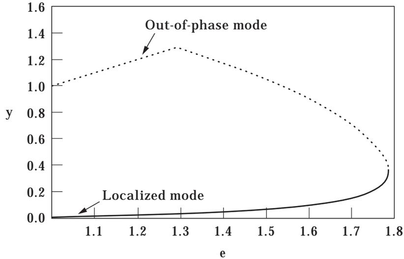
Figure 11. The bifurcation structure associated with the generation of the localized vibro-impact mode. Graphs of  $y$  vs  $e$  for each periodic solution at the time instant when  $x = -e$ : —, stable; —, unstable motions.
