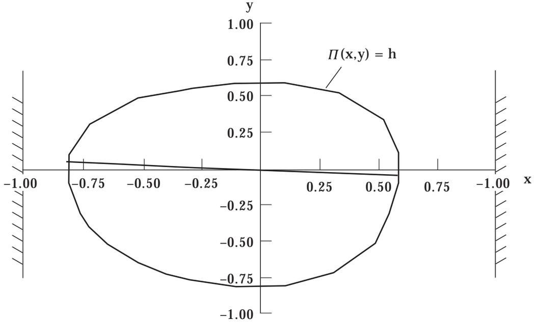
Figure 5. First order asymptotic approximation  $\hat{y}_1(x)$  to the localized nonlinear normal mode of the system with parameters  $\alpha = \beta = \delta = 1$ ,  $e = 1$ ,  $\gamma = 0.1$  and  $h = 0.26666$ .
