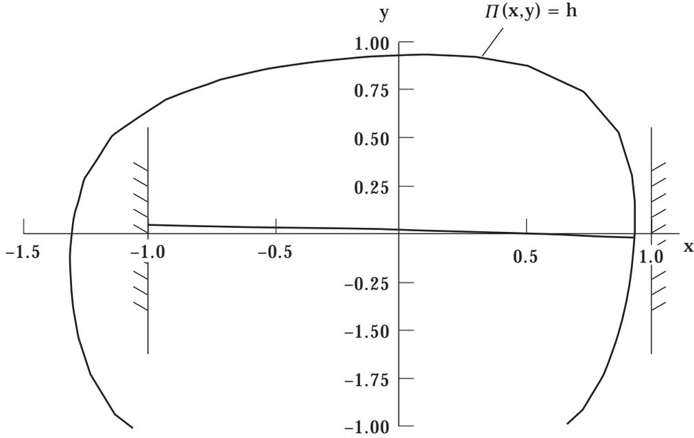
Figure 4. First order asymptotic approximation  $\hat{y}_1(x)$  to the localized single-sided vibro-impact motion with parameters  $\alpha = \beta = \delta = 1$ ,  $e = 1$ ,  $\gamma = 0.1$  and  $h = 0.933333$ .
