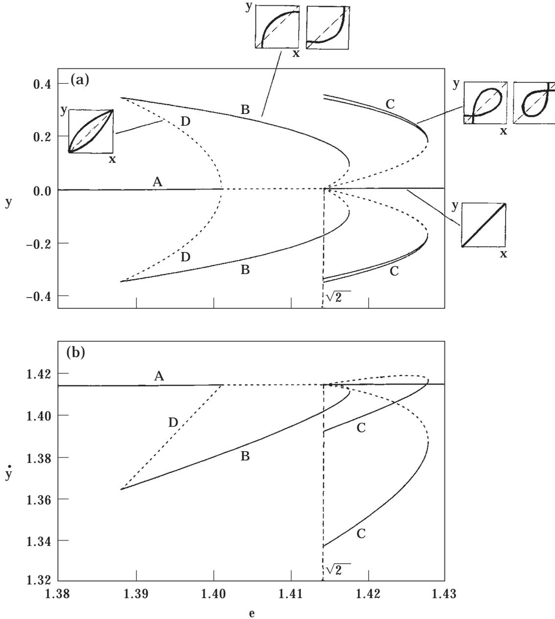
Figure 10. The bifurcation structure associated with the instability of the in-phase mode. Graphs of (a)  $y$  and (b)  $\dot{y}$  vs  $e$  for each periodic solution at the time instant when  $x = 0$  and  $\dot{x} > 0$ : —, stable; ----, unstable motions.
