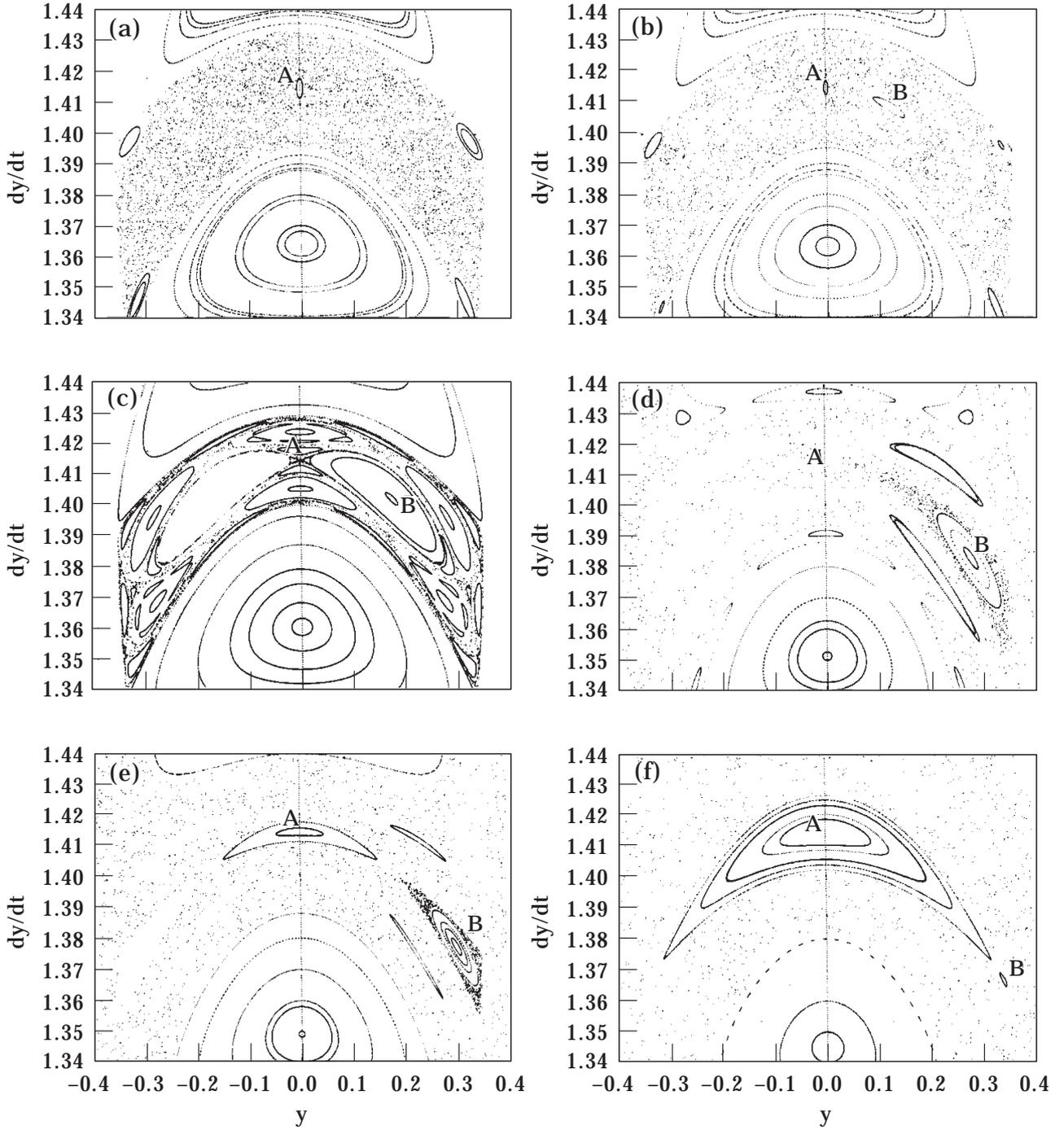
Figure 9. Poincaré maps in the neighborhood of the in-phase mode of the system with  $\alpha = 1$ ,  $\beta = \delta = 0$ ,  $\gamma = 0.1$  and energy  $h = 2$ , for clearances: (a)  $e = 1.418$ , (b)  $e = 1.417$ , (c)  $e = \sqrt{2}$ , (d)  $e = 1.402$ , (e)  $e = 1.398$ , (f)  $e = 1.390$
