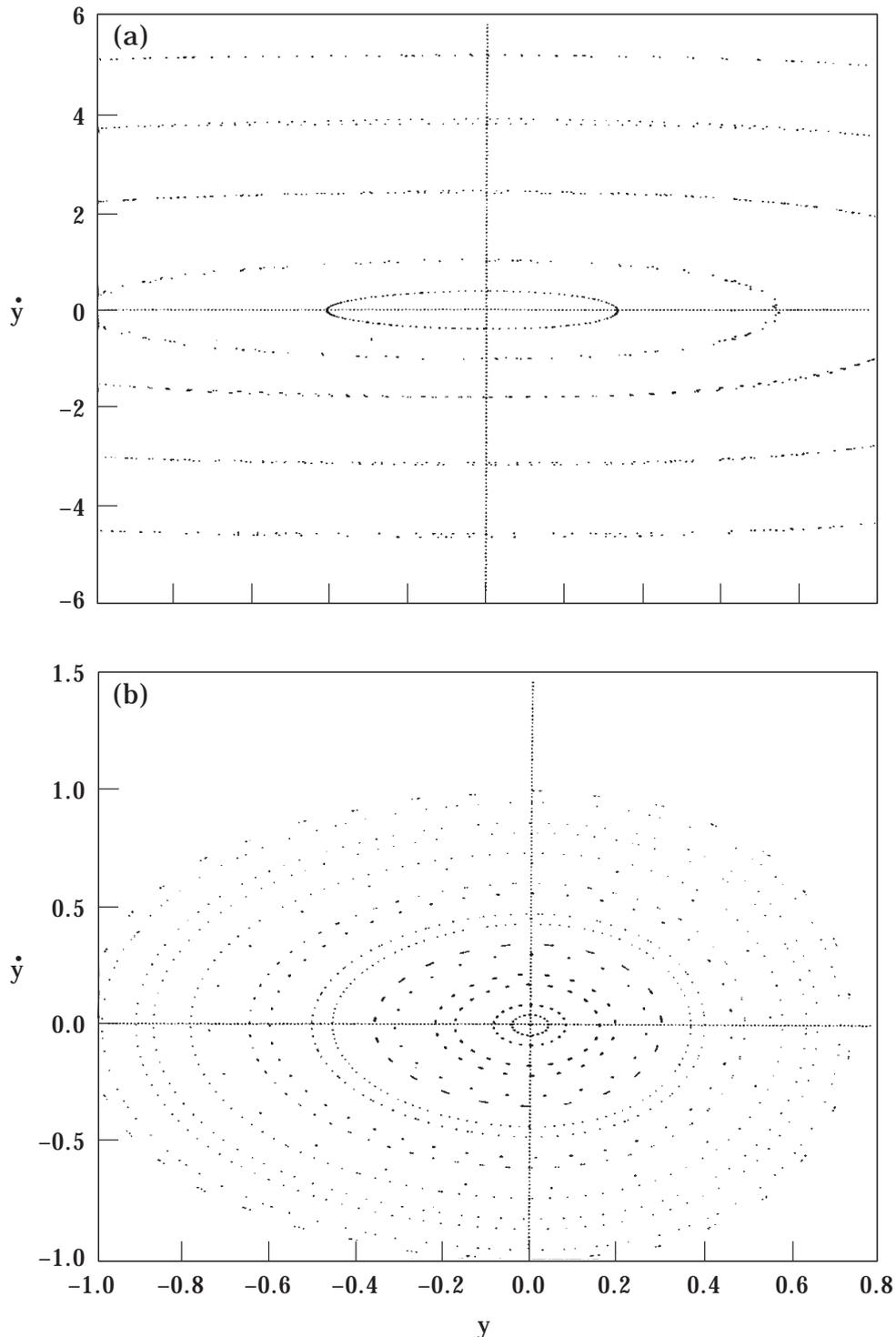
Figure 6. Poincaré map of the neighborhood of the localized vibro-impact motion of a system with  $\alpha = \beta = \delta = 1$ ,  $e = 1$ ,  $\gamma = 0.1$ , and energy (a)  $h = 18$ , and (b)  $h = 99$ .
