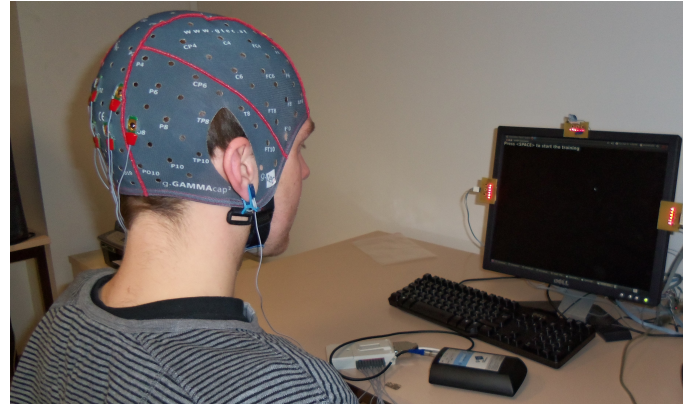
Fig. 2. Offline EEG recording. An array of 6 red LED's is used for each stimulus target. They are mounted on the sides of a 17 inches computer monitor which is used to display the experiment cues.
