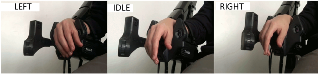
Fig. 1. The 3D touchless interface and examples of three hand poses: left, resting and right positions. The IR-sensors are in the black plastic housing on the right side of the hand and around the wrist. Another symmetrical plastic housing have been realised for left-handed users.
