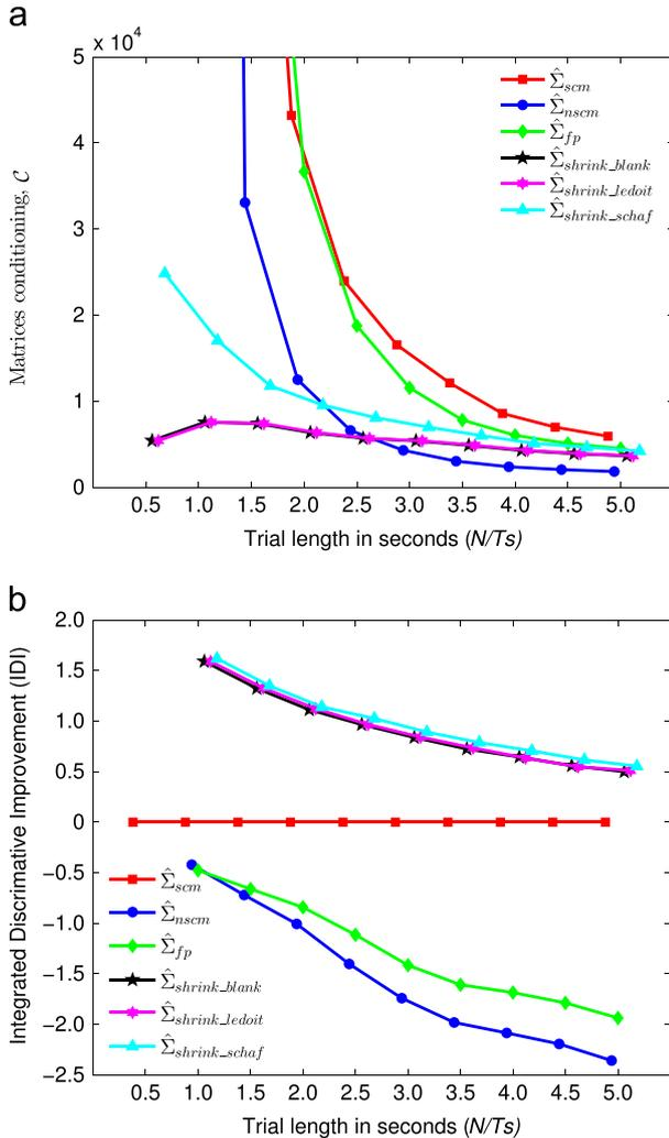
**Fig. 2.** (a) Covariance matrices condition expressed as the ratio  $C$  between largest and smallest eigenvalues for the different covariance estimators. The comparison is done for increasing EEG trial length. (b) Integrated discrimination improvement brought to the classification task by various estimators along varying trail length. The indicated IDI values are multiplied by  $10^2$ .  $\hat{\Sigma}_{scm}$  is used as a baseline.
