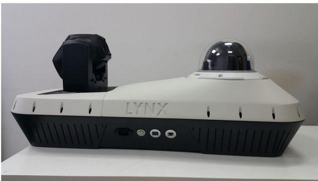
Fig. 1 Acquisition system: PTZ camera and the directional light device.
