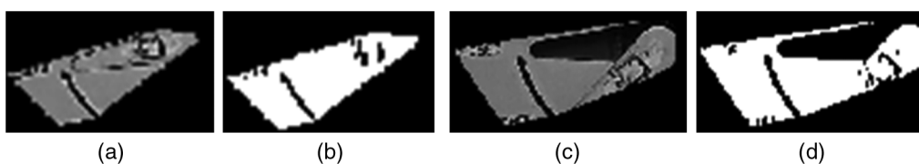
Fig. 10 Oxygen bay—region of interest (ROI) binarization by Otsu method. (a) Latched case: ROI, (b) latched case: binarized ROI, (c) unlatched case: ROI, and (d) unlatched case: binarized ROI.
