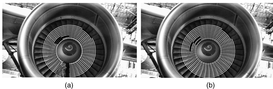
Fig. 22 Fan blades—two cases to be distinguished and circular pixel sets which are analyzed. White: circles that are extracted from the image; black: parts where the approach reported a defect, i.e., breach of periodicity. (a) Defect—presence of an object and (b) no defect.
