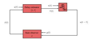
Fig. 1. State observer interconnected with delay observer
