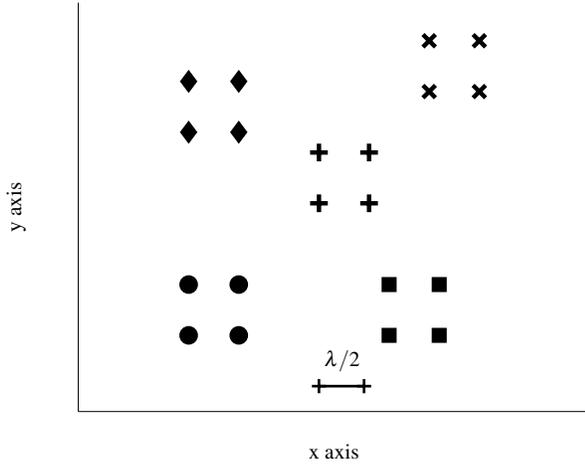
Fig. 1. Sensor position matrix
