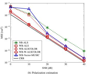
Fig. 5. MSE vs SNR - polarization diversity - seismic Rayleigh waves
