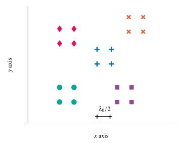
Fig. 1. Sensor position matrix - space shift diversity
