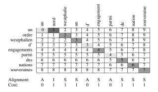
Table 1: Example (in French) of the Word Error Rate estimation between a hypothesis (on the top) and a reference (on the left).
