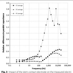
**Fig. 3** Impact of the stem contact electrode on the measured electrical capacitance of the plant–soil system. Plot of the mean relative difference between the parallel capacitance measured with a clamp and that measured with a needle, as a function of frequency, in 2T (*filled square*), 3T (*filled triangle*) and 4T (*plus symbol*) configurations. Differences are <6 % for frequencies <200 Hz in 3T configuration
