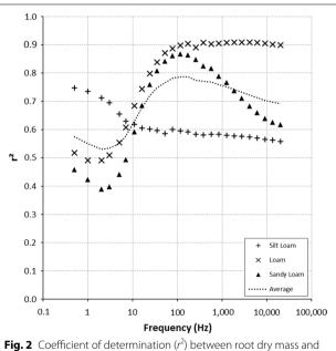
parallel capacitance, as a function of frequency. The semi-log plot was obtained from measurements for a 3T configuration, a frequency range of 0.5–20,000 Hz (log scale). Plants were grown in silt loam (*plus symbol*), loam (*times symbol*) and sandy loam (*filled triangle*) soils. The *black dots* represent the average of the three soil types. The maximum determination frequency  $f_{max}$  for average is 116 Hz
