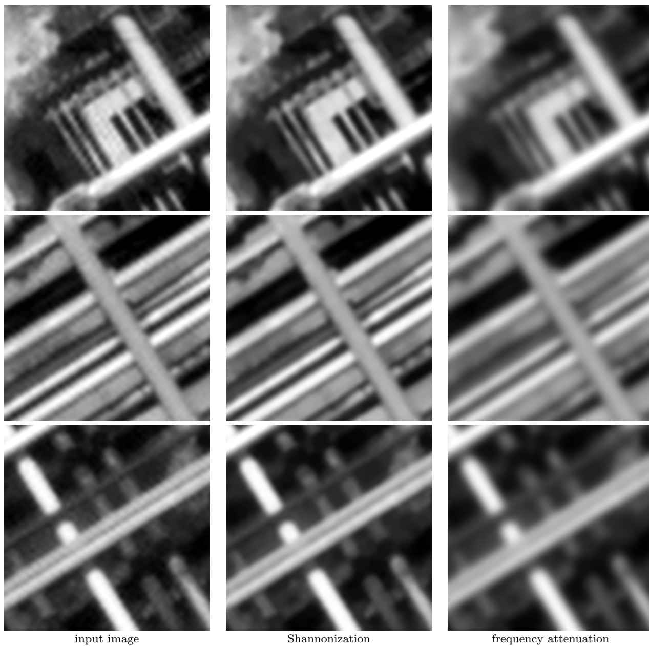
Fig. 11 Details of Fig. 10 with Shannon resampling. Different Parts of the three images of the first row of Fig. 10 are shown after Shannon interpolation. As expected, the output of the “Image Shannonizer” (middle) is well interpolable, contrary to the input image (left) on which oscillations appear. A simple frequency attenuation (right) is not efficient, since it introduces a large amount of undesired blur.
