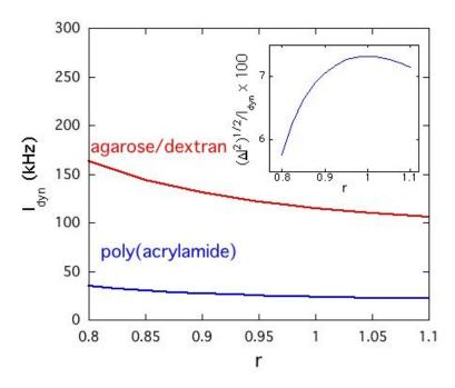
**Figure 3**. Dependence on *r* of the mean value of  $I_{dyn}$  (20 measurements) in the 100 g/l polyacrylamide hydrogel (lower curve) and for 7.5 g/l dextran in a 5 g/l agarose gel (upper curve) at 90°. Inset: variation of the normalised standard error  $(\Delta I_{dyn}^2)^{1/2}/I_{dyn}$  for polyacrylamide. The location of the extremum at r=1.00 validates the assumption that  $\beta_{\text{heterodyne}} = \beta$  for this system.
