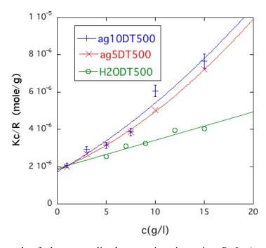
**Figure 5.** Reciprocal of the normalised scattering intensity  $R=I_{dyn}(q->0)$  from dextran (nominal  $M_w=500$  kDa) in free solution (O), and in agarose gels of concentration 5 g/l (×) and 10 g/l (+), as a function of dextran concentration.
