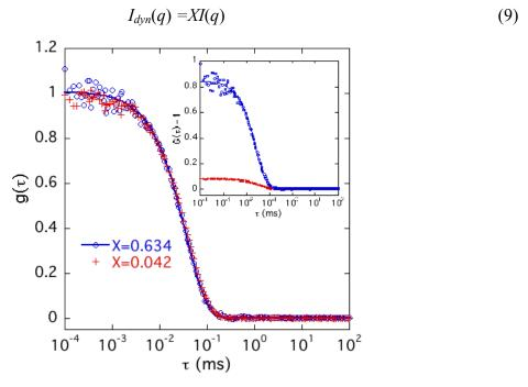
**Figure 2**. Inset: Intensity correlation functions of light scattered at 90° from a poly(acrylamide) hydrogel for two different positions of the sample (O: X=0.634, •: X=0.042). Main figure: field correlation functions  $g(\tau)$  for the same spectra calculated from Eq. 8. Continuous line is least squares fit to a simple exponential decay.
