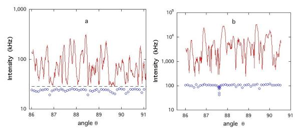
**Figure 1.** Angular dependence of intensity scattered by a) a 100 g/l polyacrylamide hydrogel without polariser, b) a 5 g/l agarose hydrogel containing 7.5 g/l dextran, with polariser. Continuous red lines are the total intensity I(q), open blue symbols are  $I_{dyn}(q)$  calculated with Eq. 9.
