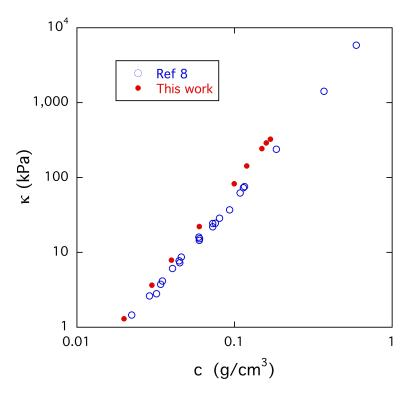
**Figure 4**. Concentration dependence of the osmotic modulus  $\kappa = c\partial \Pi/\partial c$  in polyacrylamide gels derived from Eqs. 8 and 9 (filled symbols), compared with previous results from DLS on similar polyacrylamide hydrogels made with pinhole detection geometry.<sup>8</sup>
