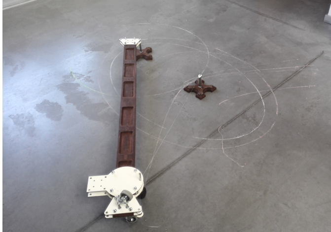
Figure 6. Prototype of ellipse-hyperbol-parabolograph, beam length 150 cm, made by the student Osvaldo Liva
