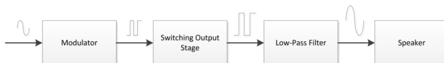
Fig. 1. Class D open-loop amplifier block diagram.
