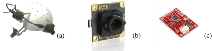
Fig. 4. Hardware used on the trials, (a) 3D printed version of part the Sphere (b) UI 1226LE-M camera from IDS-Imaging (c) 6DOF Inertial Measurement Unit.
