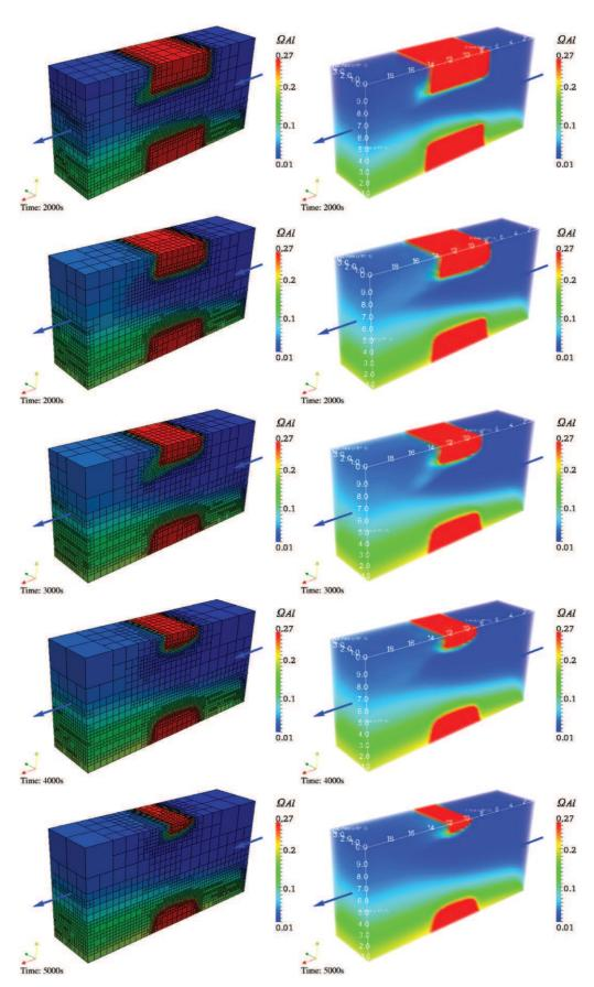
**Fig. 13.** Time evolution of the salt mass fraction  $\Omega_{Al}$  using the AMR method (left) and fine-grid solution (right). From 1000 to 5000 s, salt block is getting smaller and smaller due to dissolution. The finest mesh is moving with the solid-liquid interface for the AMR method, showing better computational efficiency. Caused by natural convection, salt plumes fluctuating with time can be found at the tail of the salt block.
