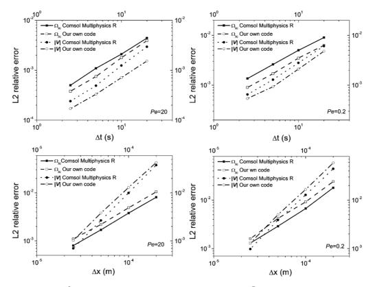
**Fig. 9.** Temporal and spatial  $L^2$ -norm relative errors of the solutions using Comsol Multiphysics<sup>®</sup> and our own code under Pe = 20 and Pe = 0.2.
