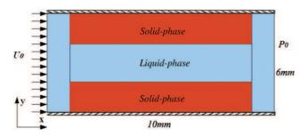
**Fig. 5.** The 2D geometry used for the simulation example. Salt blocks constitute the solid phase, water the liquid phase. The inlet (fluid velocity) is located at the left of the domain and the outlet at the right.
