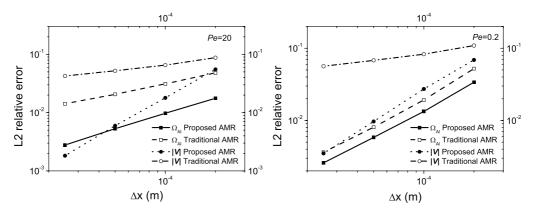
Fig. 10. Spatial  $L^2$ -norm relative errors of the solutions using the proposed AMR and the traditional AMR scheme under Pe=20 and Pe=0.2.
