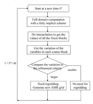
Fig. 4. Flowchart of the proposed AMR procedure.
