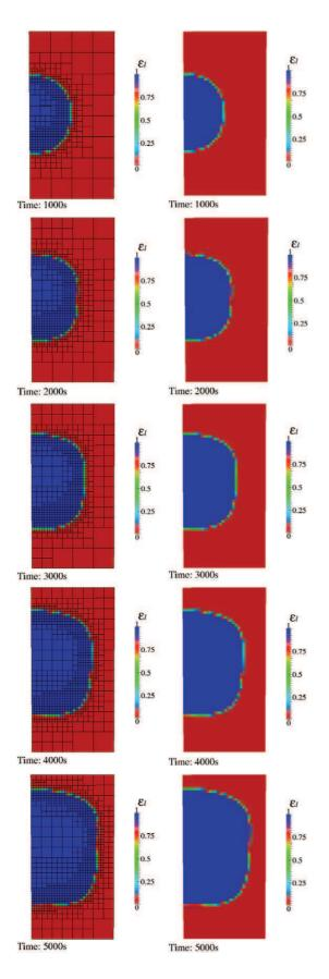
**Fig. 14.** Time evolution of the porosity  $\varepsilon_l$  at the central cross-section using the AMR method (left) and fine-grid resolution (right).
