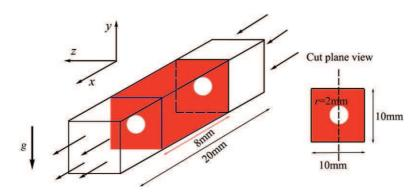
Fig. 11. Example of a 3D salt block dissolution with a cylindrical hole in the center.
