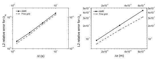
**Fig. 12.** Temporal and spatial relative errors of the mass fraction  $\Omega_{Al}$  for the 3D example using the AMR and fine grid.
