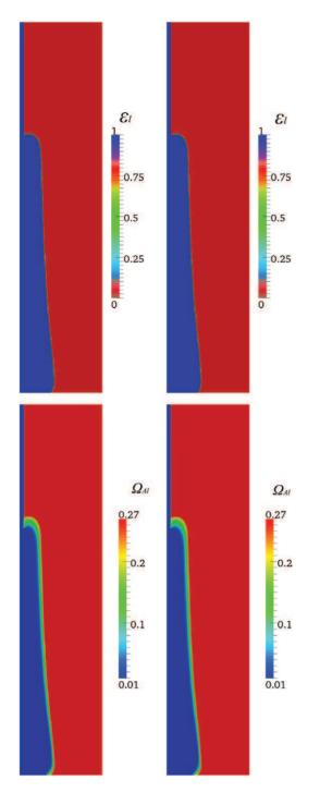
**Fig. 20.** Simulation results ( $\varepsilon_l$  and  $\Omega_{Al}$ ) using AMR method (left) and fine-grid solution (right) at time = 2 days.
