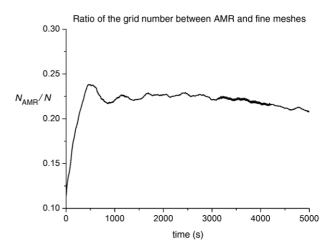
Fig. 15. The ratio of the grid block numbers between AMR and fine-grid resolutions.
