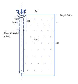
**Fig. 18.** Example of 2D-axisymmetrical dissolution using a vertical centered double-well, with vertical (inner tube) injection-inlet and production-outlet (outer tube).
