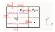
**Fig. 2.** Scheme for the calculation of the velocity flux at the grid block interface for adiacent levels.
