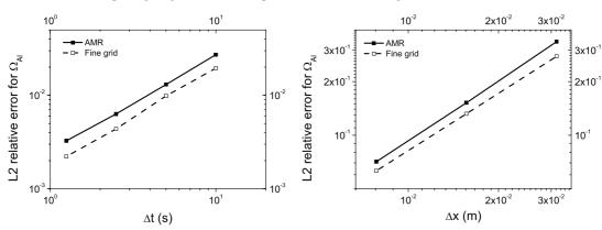
**Fig. 19.** Temporal and spatial relative errors of the mass fraction  $\Omega_{Al}$  for the reservoir-scale example using the AMR and fine grid.
