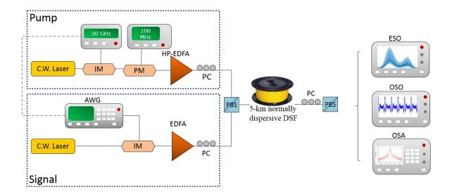
FIG. 2 Experimental setup. IM: intensity modulator, PM: phase modulator, AWG: arbitrary waveform generator, EDFA: Erbium doped fiber amplifier, PC: polarization controller, PBS: polarization beam splitter, ESO: electrical sampling oscilloscope, OSO: optical sampling oscilloscope and OSA: optical spectrum analyzer.
