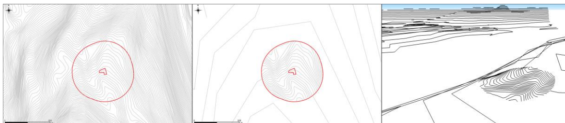
Figure 1: The refinement technique used to adapt the resolution of the Terrain model. The contour lines outside the red polygon of the studied site, have been replaced by lower resolution contour lines.
