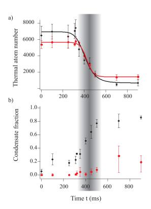
FIG. 2: a) Number of thermal atoms in  $m_s = -3$  (black diamonds) and  $m_s = -2$  (red disks) as a function of time t for a shock cooling time  $t_s = 500$  ms. b) Corresponding condensate fractions in  $m_s = -3$  (black diamonds) and  $m_s = -2$  (red disks). The shaded region highlights when both  $m_s = -3$  and  $m_s = -2$  thermal clouds are saturated, but only  $m_s = -3$  atoms condense.
