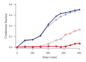
FIG. 3: Numerical results. Evolution of the condensate fractions for different values of  $a_4$  (blue diamonds:  $m_s = -3$ ; red circles:  $m_s = -2$ ). Filled markers correspond to the experimental case:  $a_4 = 64 \ a_B$  and  $a_6 = 102.5 \ a_B$  [16] where  $a_B$  is the Bohr radius. Empty markers correspond to simulations where  $a_4$  was set equal to  $a_6$  to suppress spin dynamics. A significative BEC fraction in  $m_s = -2$  is then obtained.
