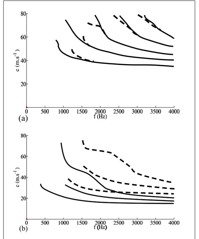
Figure 6. Phase velocity of the lowest three modes of a Fireflex cylinder of  $N = 10000$  Pa,  $\rho = 32 \text{ kg/m}^3$  (---) and of  $N = 50000$  Pa,  $\rho = 32 \text{ kg/m}^3$  (—): (a) coated with PMMA and (b) coated with steel.
