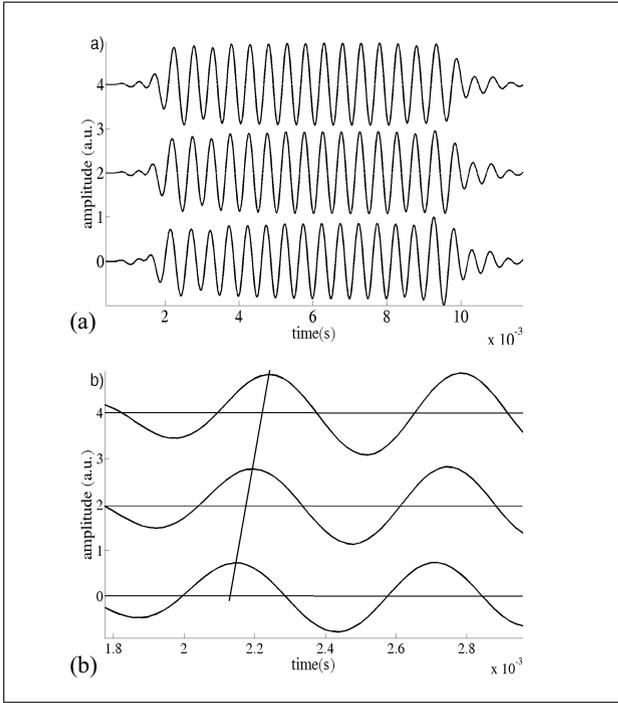
Figure 10. Example of a) response to sine bursts detected at various distances from the source (the steplength  $\Delta x$  is 2 mm) and b) zoom on the time difference between the maxima. The curves are plotted with an off-set for clarity.
