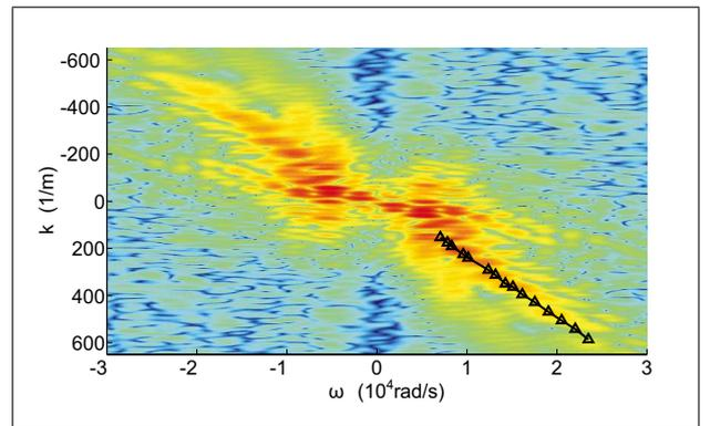
Figure 9. Example of dispersion curves from  $|S(k, \omega)|$  for a Fireflex cylinder. The line is a mode of the Fireflex cylinder that can be detected. The triangles are the experimental data extracted from the result in in Figure 12.
