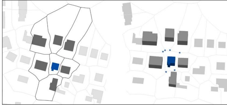
Fig. 9. Mean distance to the nearest neighbors (left) and generalized W/H ratio (right) for a given building
