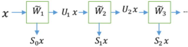
Figure 1. Scattering representation is computed by a cascade of wavelet-modulus operators \tilde{W}_m . Every \tilde{W}_m has one input and two outputs which are the invariant scattering coefficients S_m x and the next layer of covariant wavelet modulus coefficients U_{m+1} x . The latter is used for further transformations.
