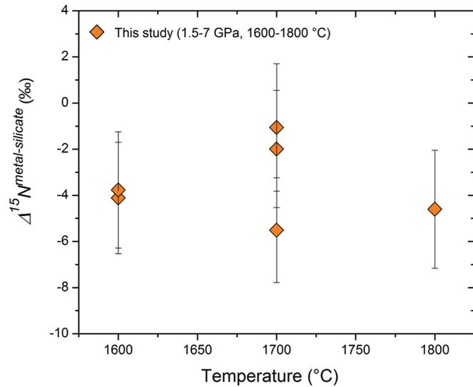
**Figure 2** Nitrogen isotope fractionation between liquid Fe-rich metal and silicate melt ( $\Delta^{15}N^{\text{metal-silicate}}$ ). Temperature has a very limited effect on  $\Delta^{15}N^{\text{metal-silicate}}$  in the  $P$ - $T$  range studied. Errors of  $\Delta^{15}N^{\text{metal-silicate}}$  are at 95 % confidence interval.
