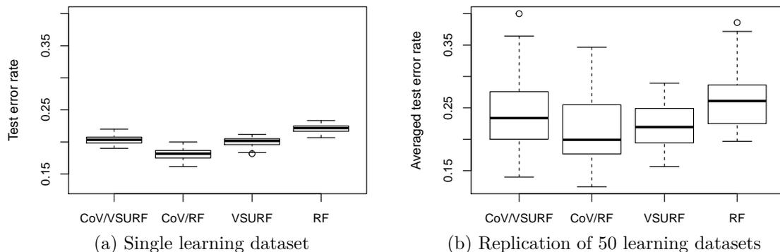
Figure 6: Comparison of test error rates with learning datasets of size  $n = 60$ . **CoV/VSURF** and **CoV/RF** correspond to **VSURF** and random forests (RF) applied on the  $K^*$  synthetic variables given by **CoV**. **VSURF** and **RF** refer to methods applied on the original 120 variables. (a) Test error rates of 100 forests trained on one learning dataset. (b) Averaged (over 100 forests) test error rates computed on 50 learning datasets.
