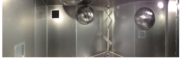
Fig. 1. 180-degree photograph of the chaotic RC (the commercial RC we modified consists in a rectangular metallic cavity of dimensions W = 2.95 \text{ m} , L = 2.75 \text{ m} and H = 2.35 \text{ m} ). Three hemispheres with a radius of 40 cm (one at the ceiling and two on adjacent walls) and a mechanical stirrer in the far corner can be seen.
