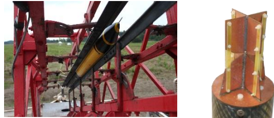
Fig. 1. Photo of the EirSpace 2015 experimental rocket (named Artemis) and its wideband bi-cone antenna [3].
