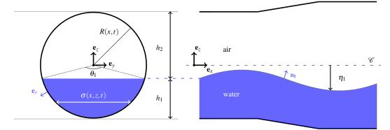
Fig. 6.1 Geometric description for circular pipes with variable cross section
