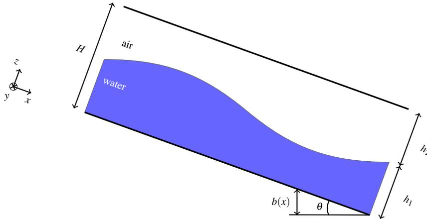
Fig. 4.1 Geometric description for sloped pipes
