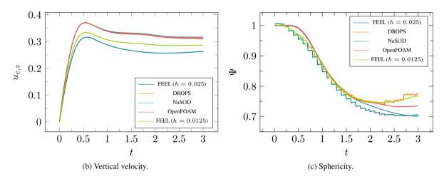
Figure 11. Comparison between our results (denoted FEEL) and the ones from [20] for the test case 2 (the skirted drop).
