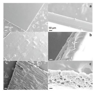
**Figure 2.** Scanning electron microscopy images of surface (left) and cross section (right) of neat EVOH (a) and its blend films containing 5 (b) and 15 (c) % digestate (D) SLP: samples E0, ED 5 and ED10, respectively, in Table 2.
