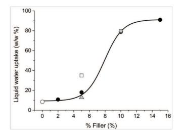
**Figure 8.** Liquid water uptake as a function of the filler content for neat EVOH (E0, white circle  $\bigcirc$ ), and its blends containing 2–15% digestate (D) SLP (black circles ●), 5% compost (CP) SLP (EC5, grey triangle ▲), and the blends containing both D and CP SLP in the same sample at total SLP concentration of 5% (ED/C2/3, white square  $\square$ ) and 10% (ED/C5/5, grey square  $\blacksquare$ ). Samples abbreviations as in Table 2.
