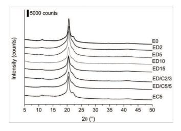
**Figure 4.** X-ray diffraction patterns relative to extruded blend sheet films. Comparison between neat EVOH (E0), and its blends containing the digestate (D) and the compost (CP) SLP. Samples abbreviations as in Table 2.
