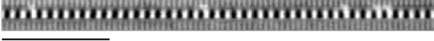
Fig. 4. 1 T tone written on a IAR = 2.6 100 Gb/in 2 sample demonstrating single track writing. The media was prepped by dc magnetizing the disk. The white wisps in between the data tracks are trench domains. The scale bar is 1 \mu m.
