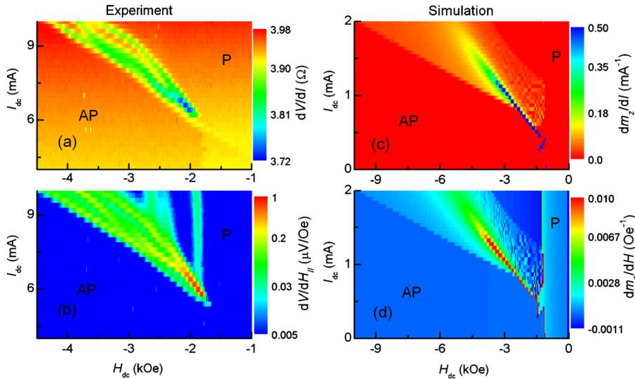
FIG. 2. (Color online) [(a) and (b)] The  $(H_{dc}, I_{dc})$  phase diagrams for the average values of  $dV/dI$  and  $dV/dH_{\parallel}$  measured by sweeping the applied dc magnetic field between 1 and  $-5$  kOe. [(c) and (d)] The  $(H_{dc}, I_{dc})$  phase diagrams for  $dm_z/dI$  and  $dm_z/dH_{\parallel}$  from the macrospin simulation in the case of the anisotropy field tilted by  $5^{\circ}$ . The regions of the P and AP states are labeled.
