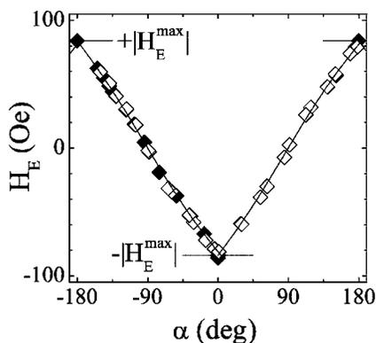
FIG. 8. Exchange-bias field  $H_E$  as a function of pinning angle  $\alpha$ . Solid and open symbols correspond to data from experiments of type I and type II, respectively. The line is the theoretical prediction.
