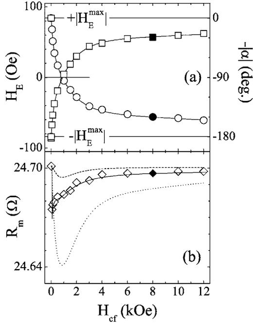
FIG. 5. (a) Exchange-bias field  $H_E$  (squares), pinning angle  $\alpha$  (circles), and (b) maximum resistance  $R_m$  (diamonds) as a function of the cooling field  $H_{cf}$  (experiments of type I), at 20 K. The open and solid symbols correspond to cases where  $\alpha$  was found negative and positive, respectively. The lines in (b) are theoretical predictions (see Sec. IV A 2 for details), those in (a) are guides to the eye.
