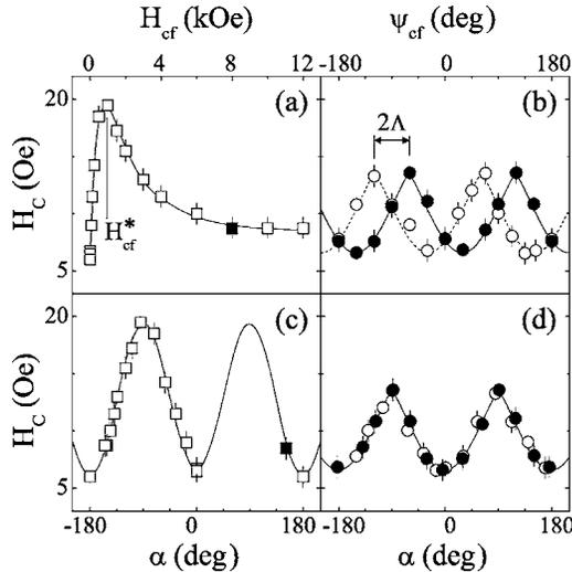
FIG. 9. Coercive field  $H_C$  as a function of the cooling field magnitude  $H_{cf}$  (a), cooling field angle  $\psi_{cf}$  (b), and pinning angle  $\alpha$  (c) (d), at 20 K. Squares and circles correspond to data from experiments of type I and type II, respectively. Open and solid symbols correspond to cases where the quenched iDW was of left handedness and right handedness, respectively. The lines are guides to the eye.
