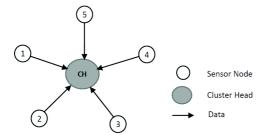
Fig. 1: Example of a cluster-star topology, show the nature of communication between sensor nodes and CH.
