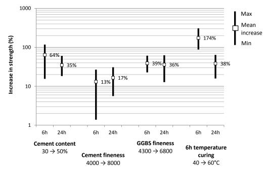
Fig. 4 Increase in strength (in %) when a given parameter went from a minimum value to a maximum value (example: GGBS fineness from 4300 cm<sup>2</sup>/g to  $6800 \text{ cm}^2/\text{g}$ )
