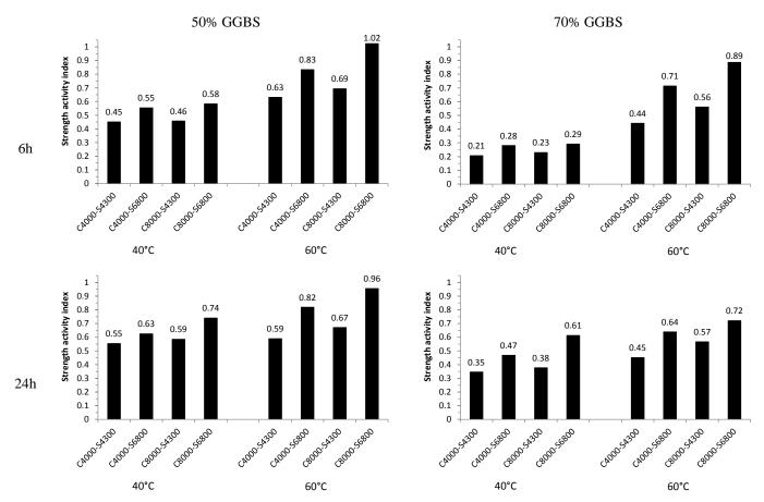
Fig. 3 Strength activity index (defined as the ratio of compressive strength of GGBS mortar and reference mortar) at 6h and 24h of mortars cured 6h at 40°C or 60°C.
