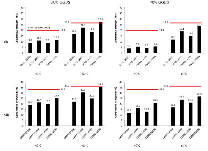
Fig. 2 Compressive strength at 6h and 24h of mortars cured 6h at 40°C or 60°C. Reference mortars contained 100% CEM I (4000 cm<sup>2</sup>/g), while GGBS mixtures (50 and 70% of fineness: 4300 or 6800 cm<sup>2</sup>/g) were made with cement of fineness 4000 or 8000 cm<sup>2</sup>/g.
