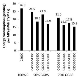
Fig. 6 Energy consumption of mortars containing GGBS. Performance energy ( $E_{performance}$ , in kWh/t/MPa) for mortars cured at 60°C (for 6h), then tests for compressive strength at 24h.
