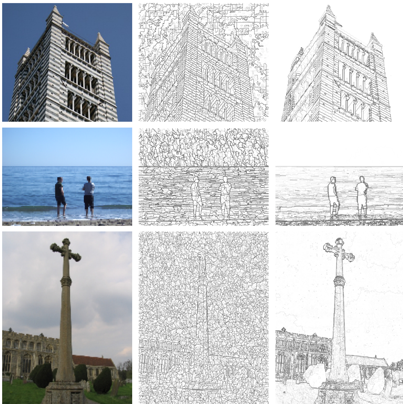
Fig. 7 First column: three color images; second and third columns: hierarchies of watersheds (saliency maps) driven by area attribute and by dynamics attribute respectively.
