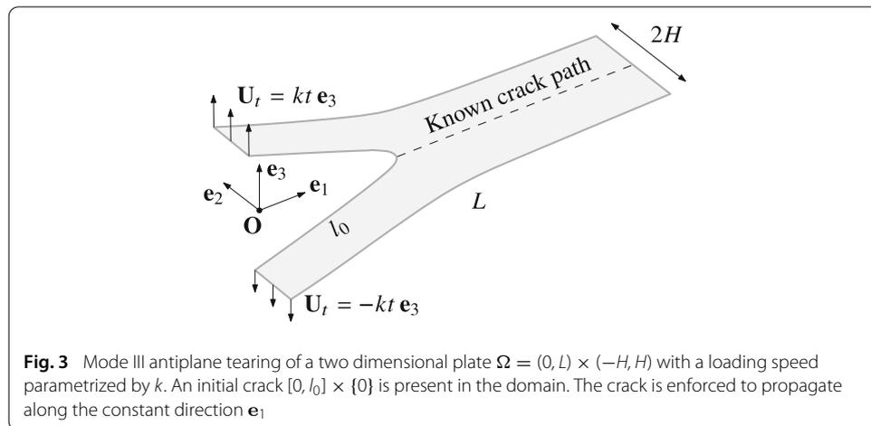
**Fig. 3** Mode III antiplane tearing of a two dimensional plate  $\Omega = (0, L) \times (-H, H)$  with a loading speed parametrized by  $k$ . An initial crack  $[0, l_0] \times \{0\}$  is present in the domain. The crack is enforced to propagate along the constant direction  $\mathbf{e}_1$
