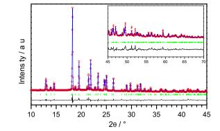
**Fig. 1.** Final Rietveld refinement of X-ray diffraction pattern of *p*-synephrine obtained at 294 K. Blue line: experimental pattern, empty red circles: calculated pattern, green vertical bars: peak positions, black line: residual XRPD patterns. The insert corresponds to the scale for the data between 45° and 70° magnified 15 times. (For interpretation of the references to colour in this figure legend, the reader is referred to the web version of this article.)
