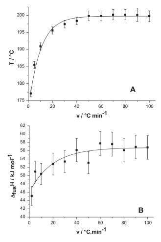
**Fig. 5.** Temperature (A) and enthalpy (B) of melting of *p*-synephrine as a function of the heating rate.
