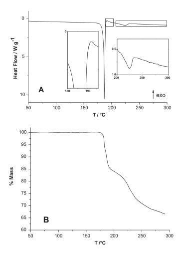
**Fig. 3.** DSC (A) and TGA (B) curves of *p*-synephrine recorded at  $5 \circ \text{Cmin}^{-1}$ . The inset of panel A corresponds to the zoom of the degradation region between 175 and 300 °C.
