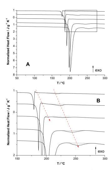
**Fig. 4.** (A) Selected normalized DSC curves at 2, 5, 10, 30, 50 °C min<sup>-1</sup> (from top to bottom). (B) Zoom of the DSC curves from (A) highlighting the endothermic heat effects due to degradation. Red arrows indicate the degradation shift to higher temperatures. (For interpretation of the references to colour in this figure legend, the reader is referred to the web version of this article.)
