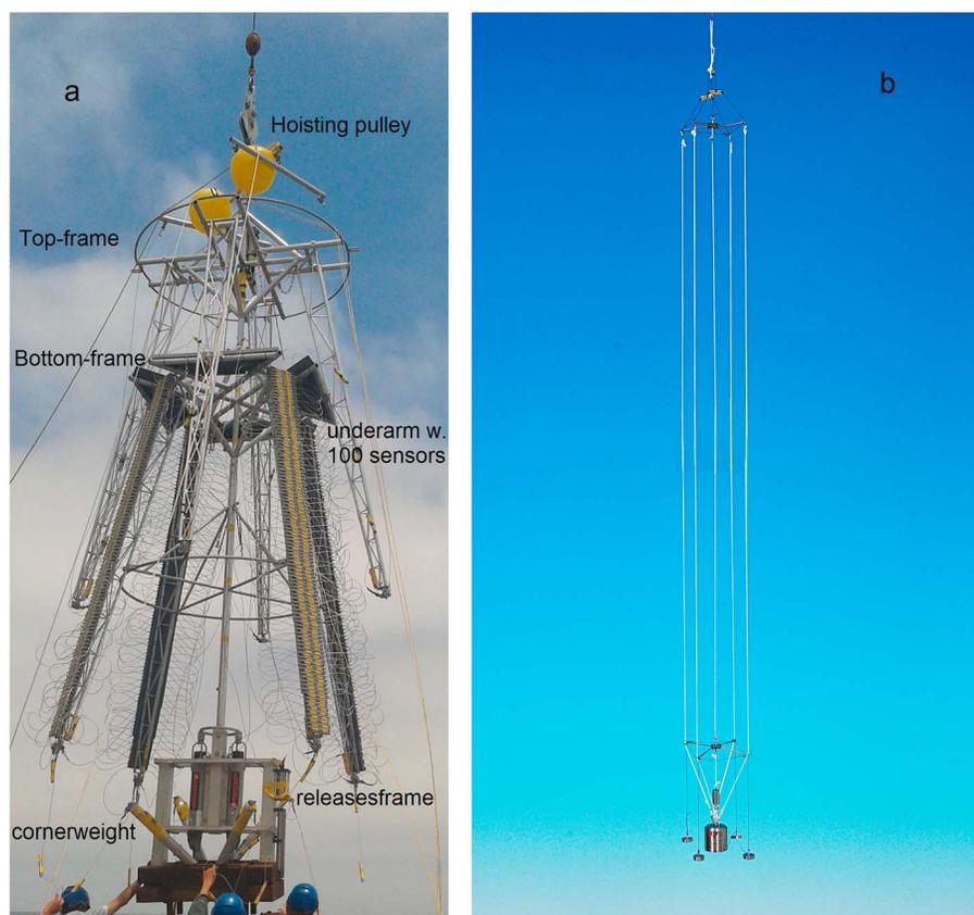
**Figure 1.** (a) Compacted 3-D mooring array of temperature sensors just before deployment in the ocean. (b) Model of the unfolded array to scale.
