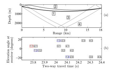
FIG. 2. (a) Example of propagation with four eigenrays between a sonar at 200 m in depth and a target at 400 m in depth and 18-km range. (b) Elevation angles at the receiver as a function of the two-way travel time for the two-way ray propagation of the top panel. In each box, the number of the left represents the ray path used between the sonar and the target, and the number of the right represents the ray path used between the target and the receiver array.
