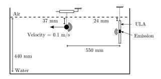
FIG. 6. Set-up of the experimental water-filled tank. The experiment was composed of a vertical uniform linear array (ULA) with 64 transducers, and a moving spherical target.
